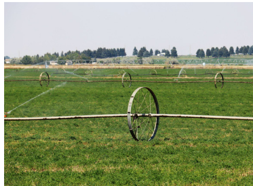
Figure 5 - Wheel-line sprinkler system with a modern pivot sprinkler in the background, both examples of field-conveyance systems on the Minidoka Project, summer 2021, Laura Woodworth-Ney, Photographer.
