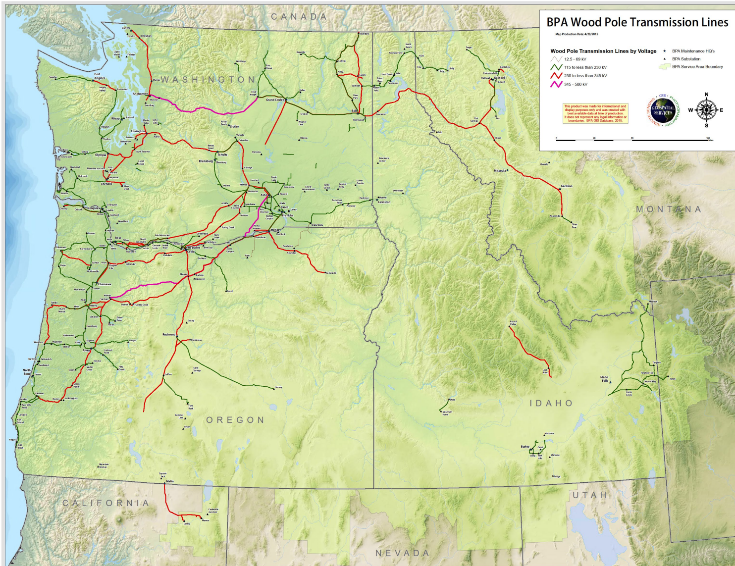
Figure 77. BPA's Wood Pole Transmission Lines delineated by voltage.
